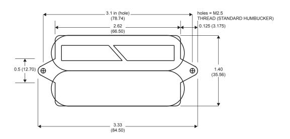
NOTE: Same cover used on both HB and SC versions. Dummy cover used on HB version same dimensions as driver cover
